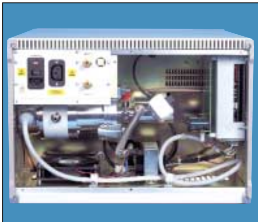
Option - Turbo Pump, 60 Litres per second backed by a Diaphragm Pump (Oil Free)
